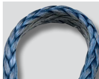
Example of 12-strand with compression
