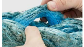
Inspect for pulled strands
