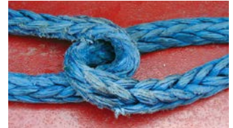
Eye-to-eye splice connection.
