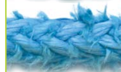
Severely abraded 12-strand rope
